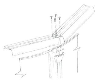
P.No.0514 1/4"x28mm Truss Head Screw
