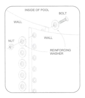
DO NOT FASTEN THE WALL WITHOUT USING THE REINFORCING WASHERS! FAILURE TO USE REINFORCING WASHERS AS INSTRUCTED WILL CAUSE WALL TO SPLIT WHEN POOL IS FILLED. THIS CAN CAUSE SERIOUS PROPERTY DAMAGE AND/OR BODILY INJURY.
